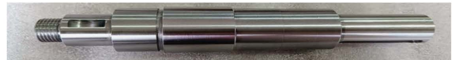
Shafts – Oil seal Bearing – Zero Lead
